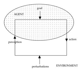
The feedback loop characterizing a control system or agent has the following basic components (see picture):
